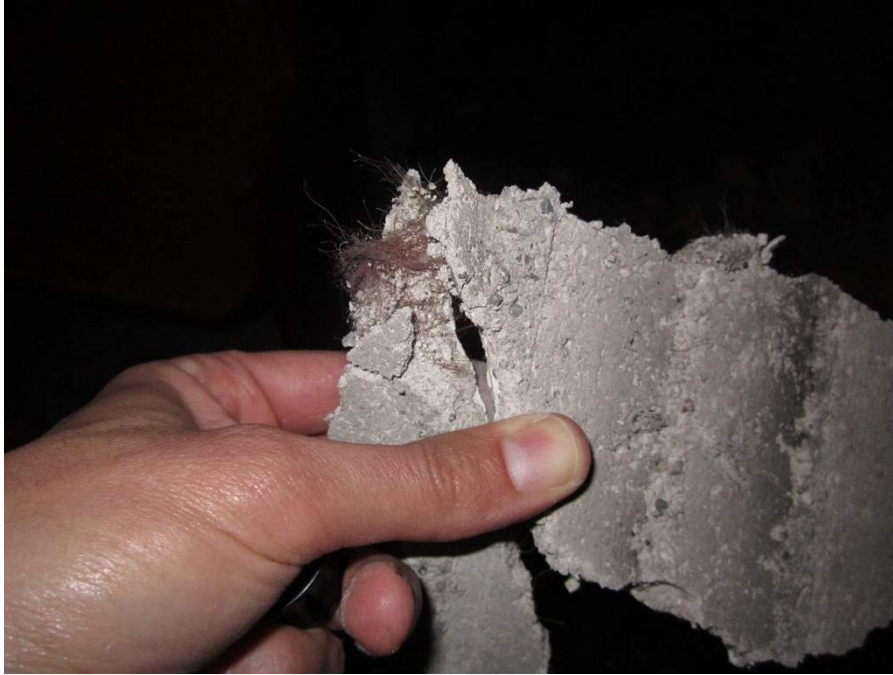
Figure 8. Fibrous material, likely plant fibers, in plaster.
